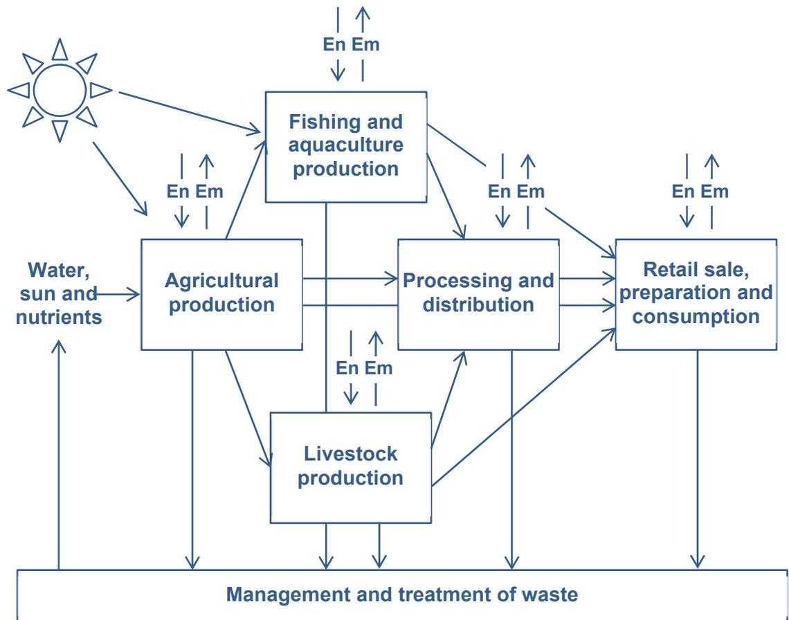
Figure 2.1 Diagram of the sectors of activity in the human food chain (En = energy; Em = emissions). Compiled by: X. Flotats
