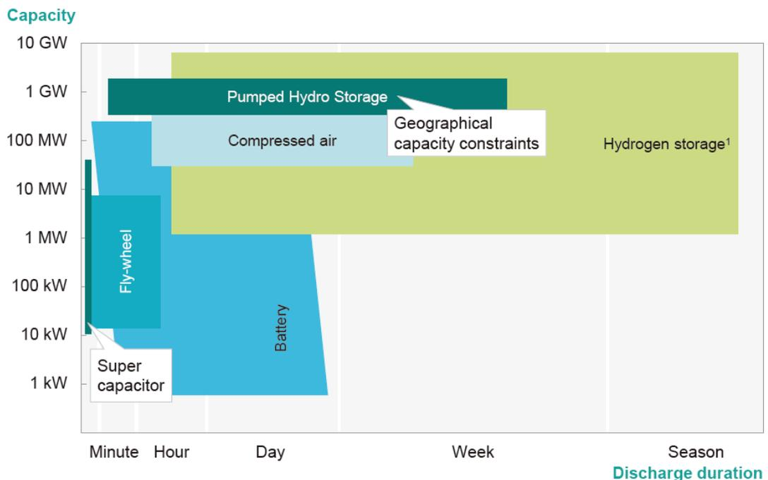
Figure 7.1 Fields of application of energy storage systems by amount of energy and storage time [Hydrogen Council-2017]
