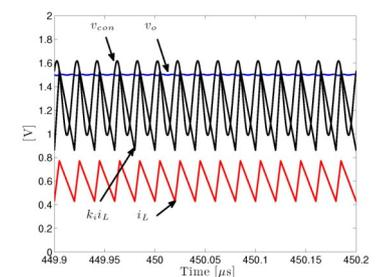
Time-domain waveforms of the state variables in a CMC buck converter without (top) and with (bottom) LC divider chaos controller. Stability is observed without using compensating ramp and output voltage ripple is reduced
