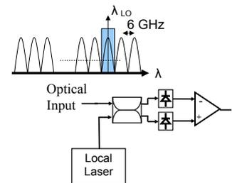
The design avoids the use of external cavity lasers and of optical hybrid
