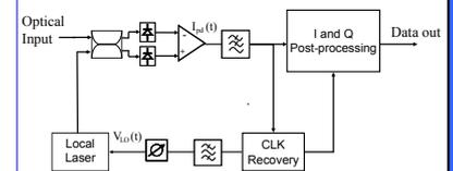
The I&Q orthogonal components of light are forward processed in switched time differentially
