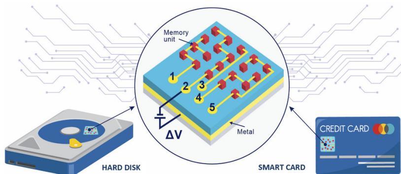
Fig. 1: Schematic drawing of the voltage-actuated multi-element memory chips that we develop to be integrated in energy-efficient hard disk drives or anti-counterfeiting technologies.
