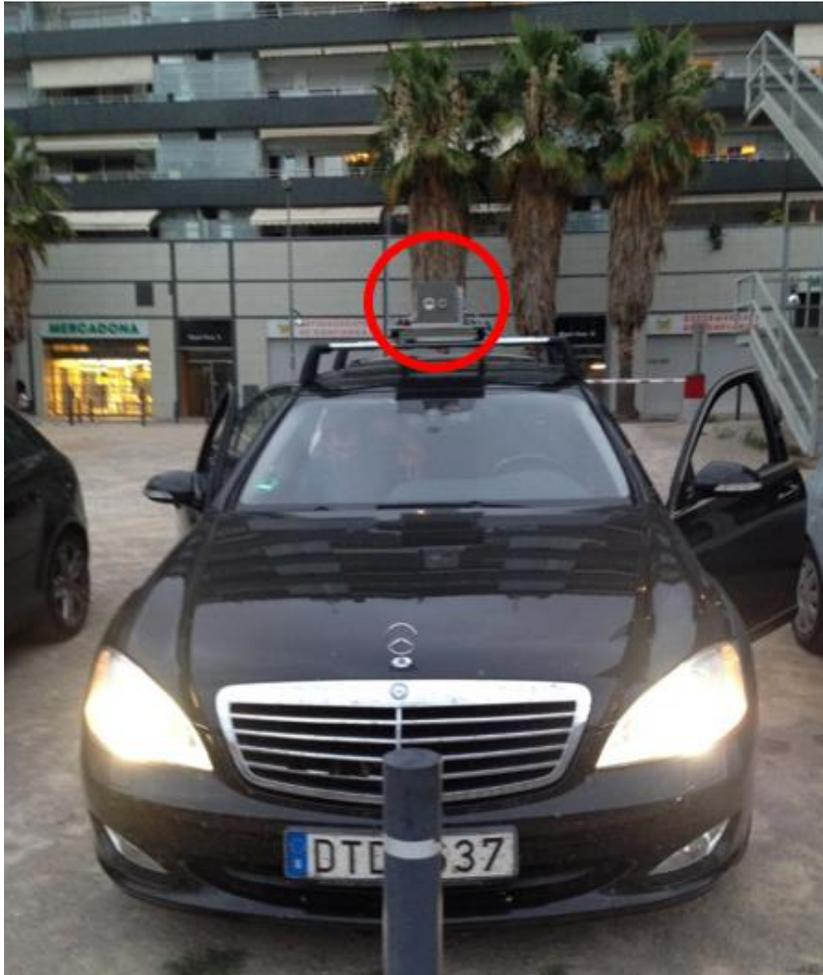
Co-located Lidar & cameras
