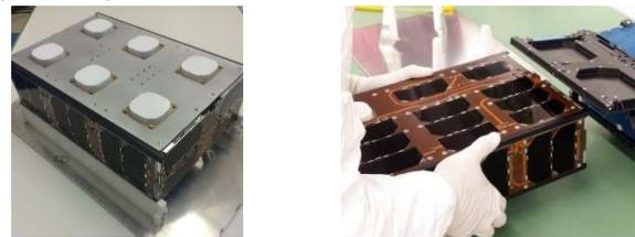
**Fig. 5.** <sup>3</sup>Cat-2 nadir looking antenna array (left), and <sup>3</sup>Cat-2 during integration in the DuoPack deployer at ISIS premises.
