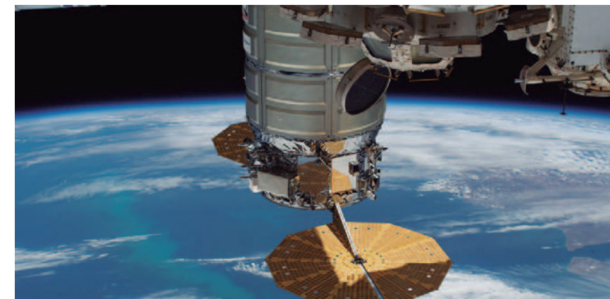
The U.S. Cygnus space freighter and its cymbal-shaped UltraFlex solar arrays. (Mark Garcia/NASA)
