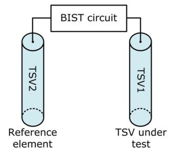
**Behavior comparison between the TSV under test and a reference element**
