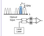
The design avoids the use of external cavity lasers and of optical hybrid
