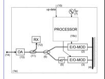
ONU modulates the downstream light after shifting it slightly in the optical spectrum, to avoid the bidirectional down/up crosstalk
