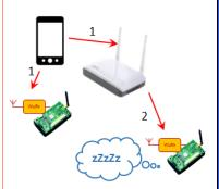
Wi-Fi Access Point and sensor devices controlled by a smartphone through Wi-Fi communications
