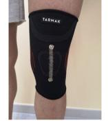
Textile strain sensor used as a goniometer on one knee to measure the degree of mobility of a patient
