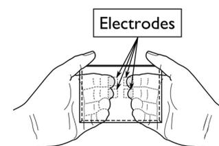
The ECG and a proximal and two distal IPGs are recorded with four electrodes
