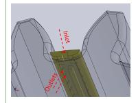
Micro channels technology is used to distribute the lubricant into gear contact area
