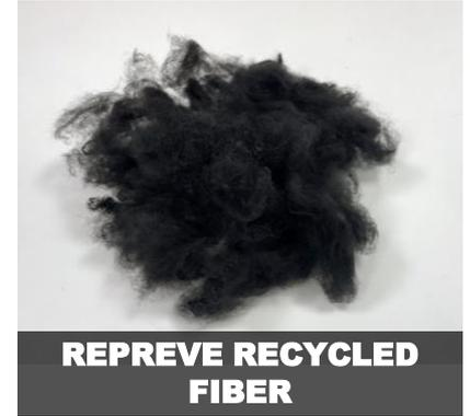
Resin is melted and made into REPREVE staple fiber
