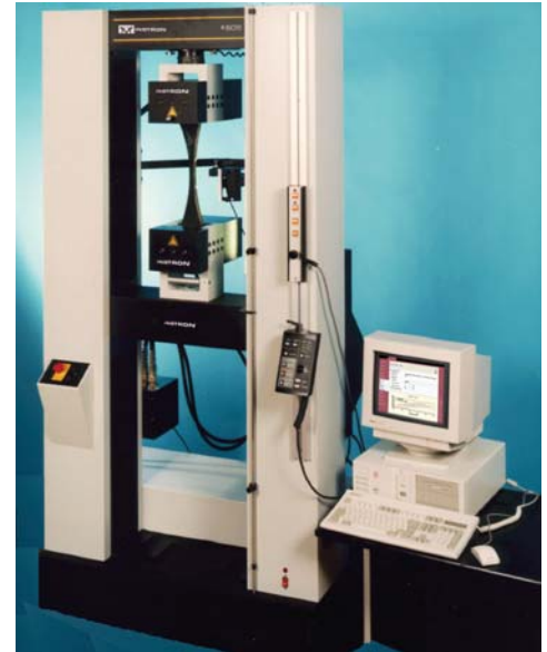
▲ An Instron 4505 testing frame with 5500 series electronics and Bluehill 2 software
