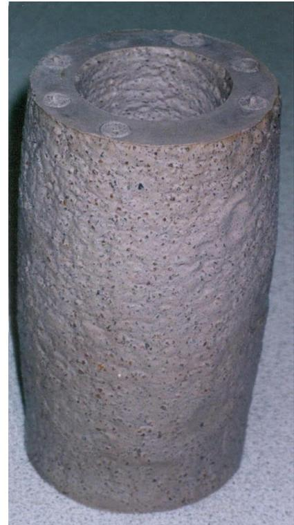
Fig. 6 Hollow Cylinder Test Specimen
