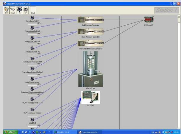
Fig. 1 Object display showing a GDS SS-HCA arrangement
