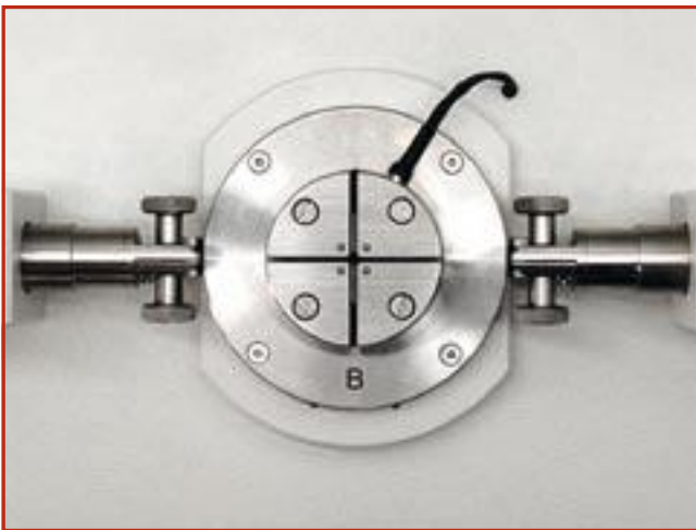
Folding head with temperature sensor
